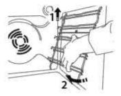
Pull the heating element out a little and lower it.
