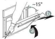
Refit the door by moving it towards the oven, aligning the hooks of the hinges with their seating and securing the upper part onto its seating. 4. Lower the door and then open it fully. Lower the catches into their original position: Make sure that you lower them down completely.
