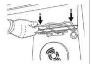
To reposition the heating element, lift it up, pulling it slightly towards you, making sure it comes to rest on the lateral supports.
